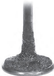
Intake Valve before P.i. Treatment
