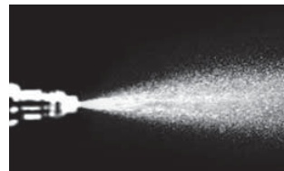
Injector spray pattern after P.i. treatment.
