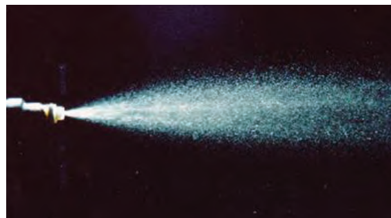
Picture C - Injector spray pattern after P.i. treatment
