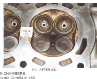
Picture H - Combustion chamber after P.i. treatment
