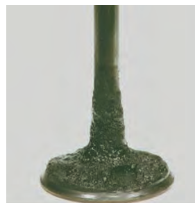
Picture D - Intake valve before P.i. treatment
