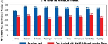
The ASTM D975 diesel fuel standard specifies a wear scar below 520  $\mu m$  in ASTM D6079 testing, while the Engine Manufacturers Association (EMA) specifies a wear scar below 460 um. Testing reveals AMSOIL Diesel Injector Clean provides significant lubricity improvement in diesel fuels found across the U.S., delivering improved wear protection
