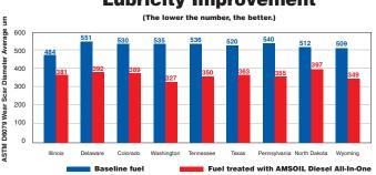
The ASTM D975 diesel fuel standard specifies a wear scar below 520  $\mu m$  in ASTM D6079 testing, while the Engine Manufacturers Association (EMA) specifies a wear scar below 460  $\mu m$ . Testing reveals AMSOIL Diesel All-In-One provides significant lubricity improvement in diesel fuels found across the U.S., delivering improved wear protection.
