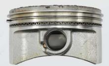
The piston and rings are virtually free of deposits and wear after 500 hours of severe-service testing in the Kawasaki\* FX 730 V engine.
